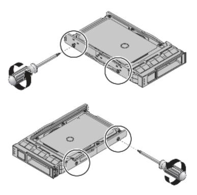
2. Install the new SSD into the drive carrier that is compatible with the DE2-24P Drive Enclosure. Use the extra drive carrier and the screws provided in this kit.
